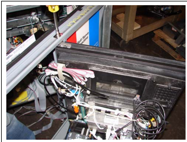
Figure 5: Securing the FlexPay EMV CRIND Door
