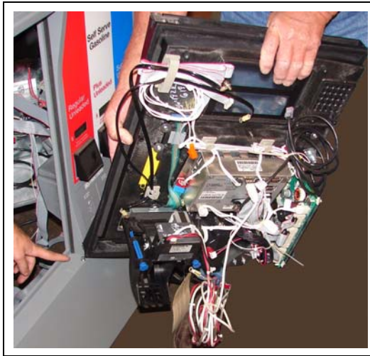
Figure 4: Mounting Location of the FlexPay EMV CRIND Door
