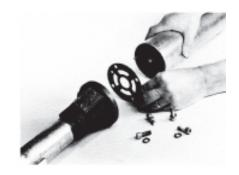
TO RE-ASSEMBLE: Replace gasket, align dowel pin, draw in place with cap screws.
