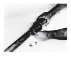
Remove the four screws holding motor to the discharge head.
