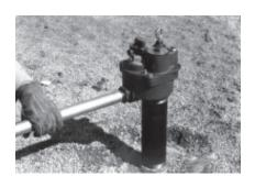
4. Line up discharge outlet. Turn in "tightening" direction only.
