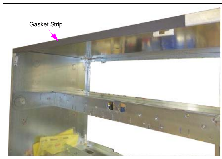
Figure 7: Gasket Strip Installed
