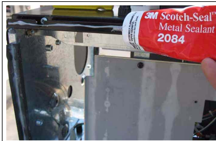
Figure 10: Application of the Sealant - Front Surface
