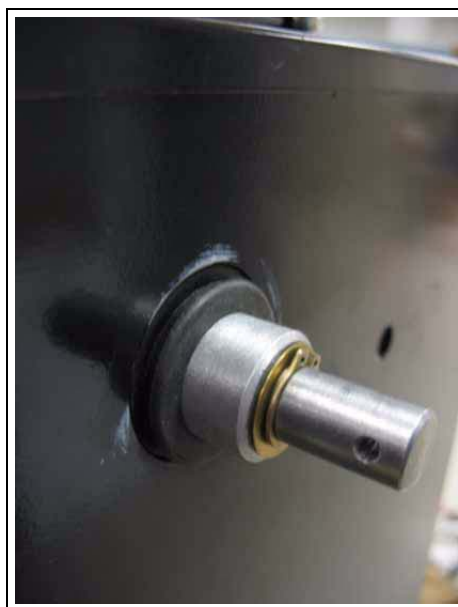
Figure 6: Reset the Shaft and Grommet
