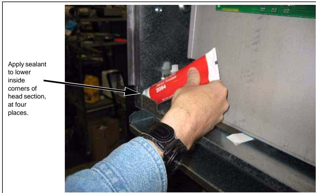
Figure 9: Application of the Sealant - Bottom Corners
