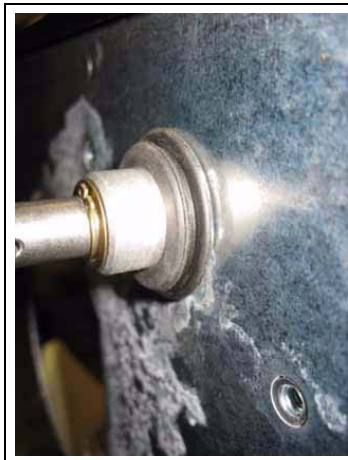
Figure 5: Installation of the Grommet Over the Shaft
