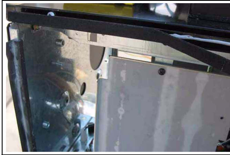
Figure 11: Application of the Gasket Strip
