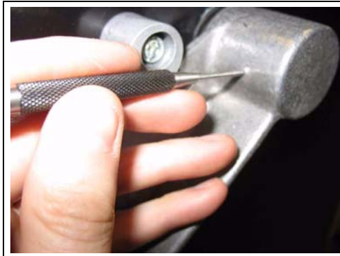
Figure 3: Removal of the Reset Handle
