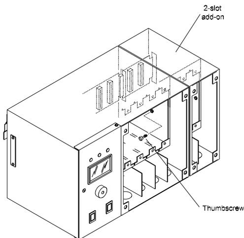
**Figure 3 Securing the 2-slot add-on**
