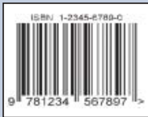
Information on a 1-D bar code is stored horizontally in one dimension as shown above.
