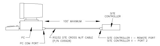
NOTE: If you are installing PC/CFN on your Gasboy Site Controller III PC, you must connect Site III Port 4 to Comm 1 or Comm 2 using a C05995 cable and a C01633 adapter to enable communication between the PC/CFN software and the Site Controller III.
