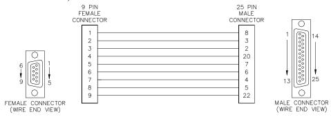
NOTE: Most PCs that use a 9-pin RS-232 connector for serial communication also include a 25-pin converter cable assembly. This cable (or one purchased from a store that supplies PC parts) should provide the necessary cabling conversion. A converter is supplied with a C04654 cable.
