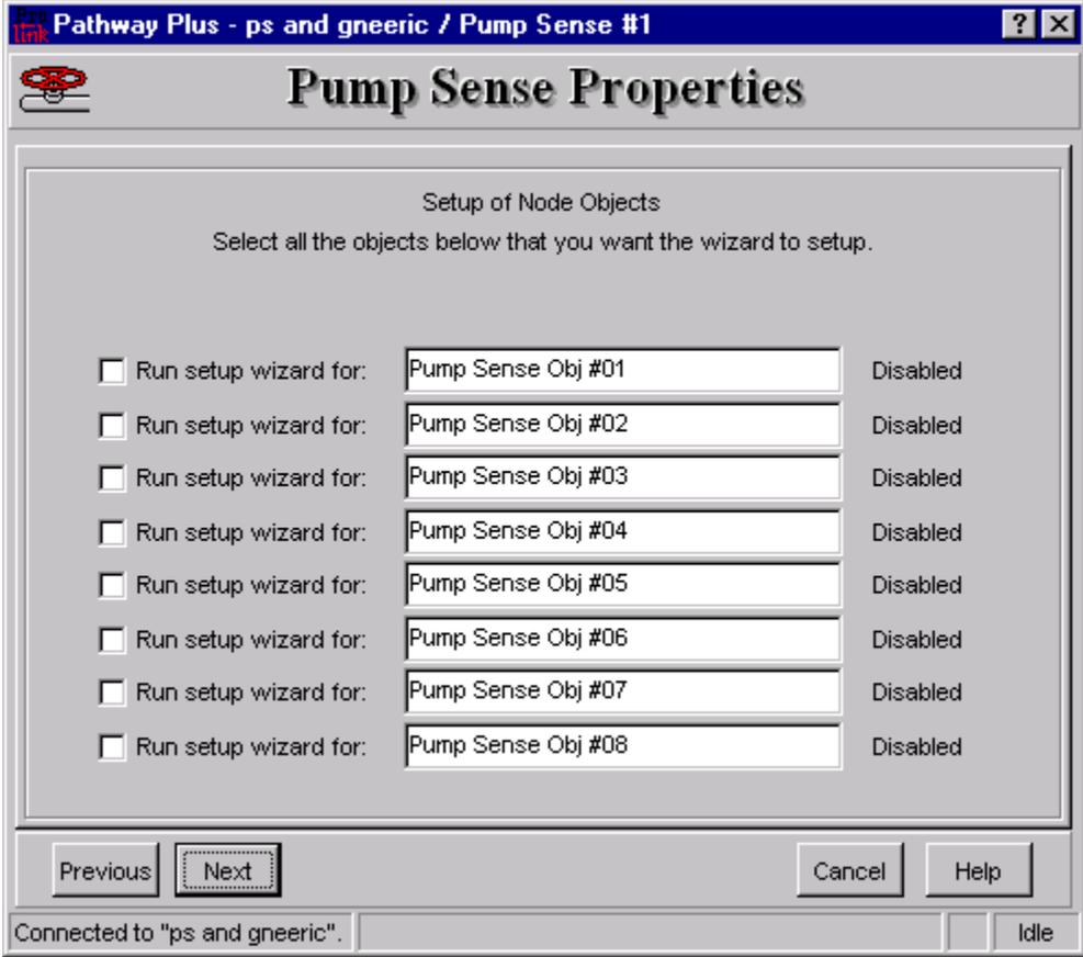
This section allows the user to select which type of objects that they want the Prolink Setup Wizard to configure at this time.
