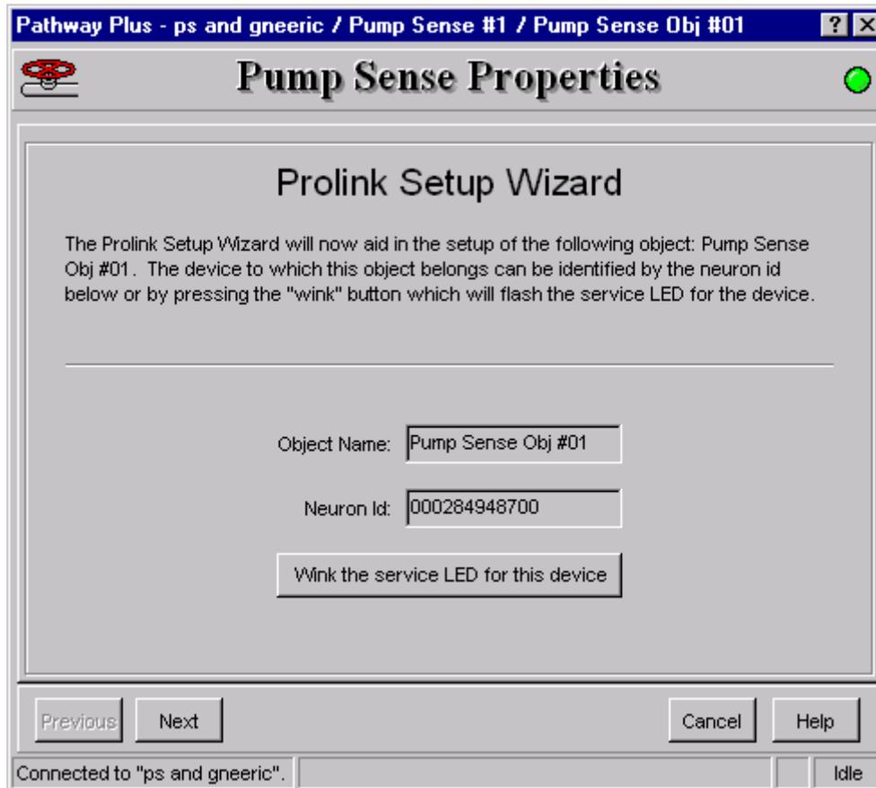
**Wink:** Click on this button to blink the service LED on the node. This is helpful in situations where there is more than one network card of the same type installed in the same chassis. Blinking this LED will identify the specific card that is being configured.
