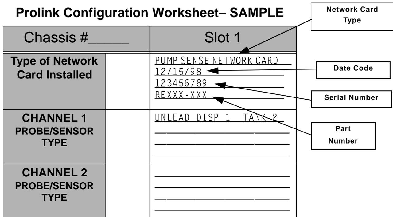
Figure 2.4 Pump Sense network card required information
