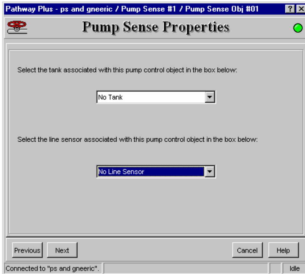
**Select Tank:** If a tank gauge card such as the Mag card, Sonic card, or Generic Tank card is installed in this Prolink you will need to select the tank that is associated with this object.
