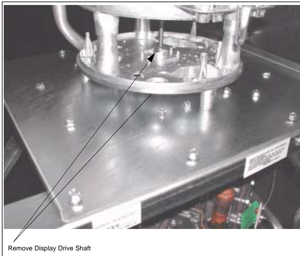
Figure 6: Drive Train Shaft Removal
