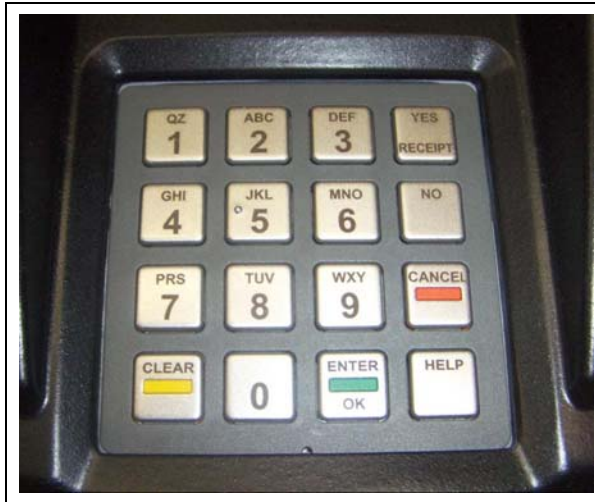
Figure 4: Properly Installed Keypad
