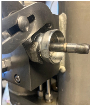
Figure 11. Outlet Valve Assembly Removal
