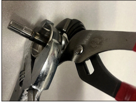
Figure 13. Separating the Outlet Valve Body from the Valve Seat
