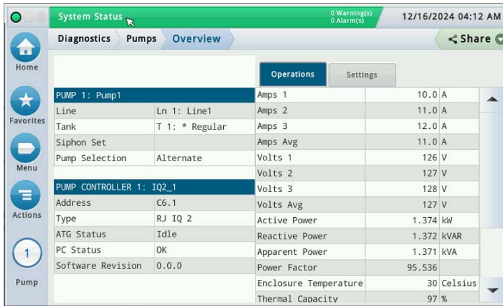
Figure 33. Example Pumps Overview Screen
