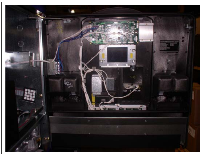
Figure 19: Upgraded FlexPay EMV CRIND Door
