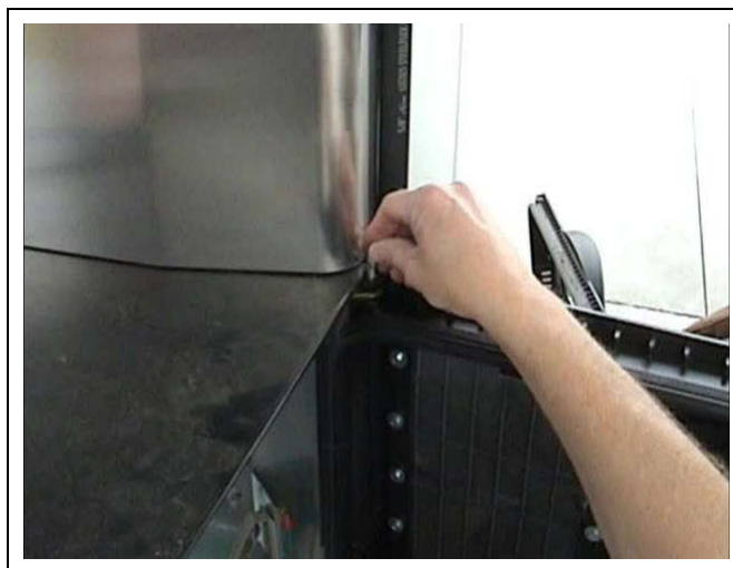
Figure 13: Installing FlexPay EMV CRIND Door
