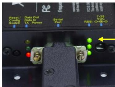
Each XTend Modem will show a green signal when polled, XStream modems do not have signal lights.
