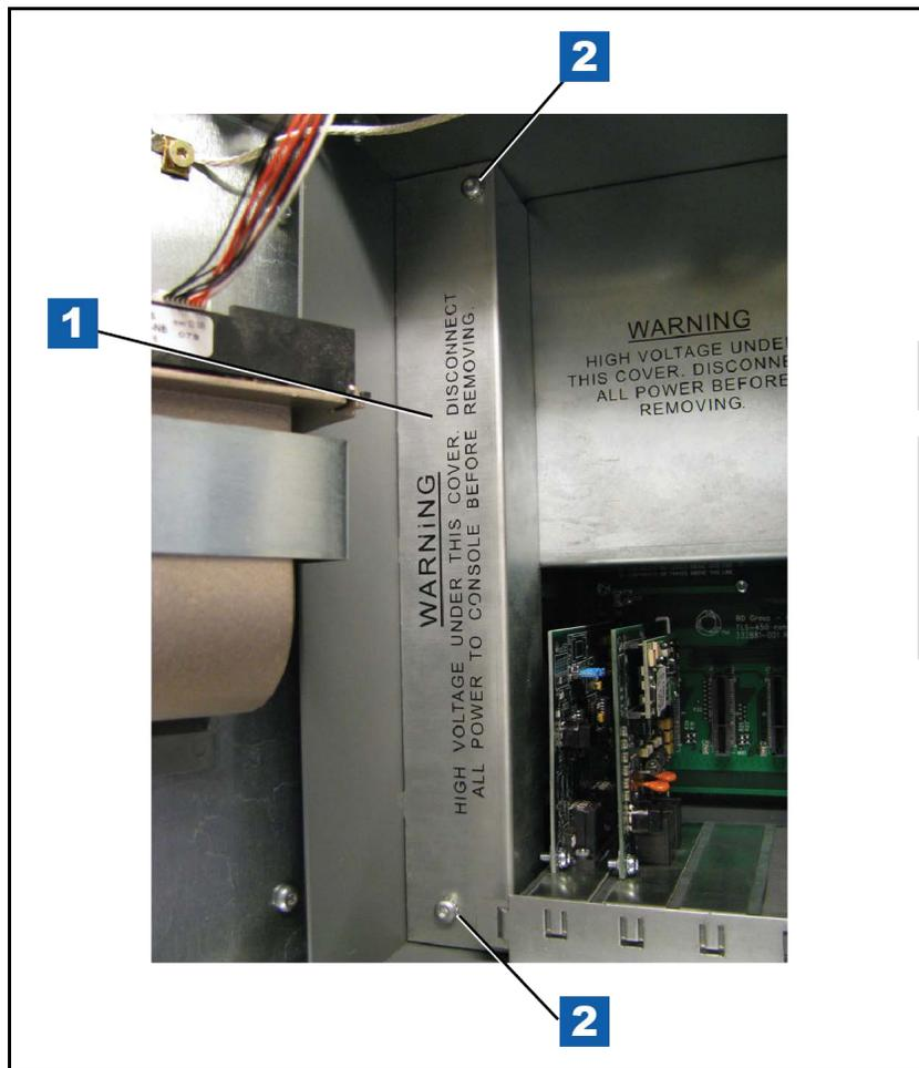
Figure 9. Remove AC Channel Cover
