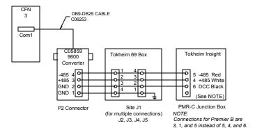
Connect the power supply (part# C05440) to the 9600 converter and plug it in.
