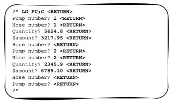
**5** Type LO TA;C to load the system's initial quantity, product code and reorder level for each tank (tank inventory) (Figure 13-16).
