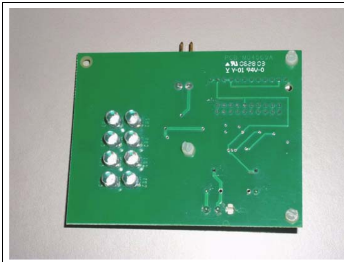
Figure 11: Satellite Indicator PCA (Front View)
