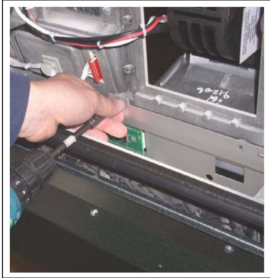
Figure 10: Removing the PPU Panel
