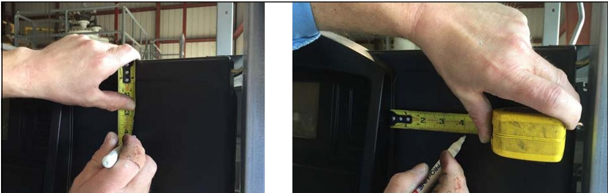
3. On the outside of the door, mark the center of the intended mounting hole with the marking pen. (It is preferable to drill the mounting hole from the outside to minimize damage to any front panel paint/graphics.)
