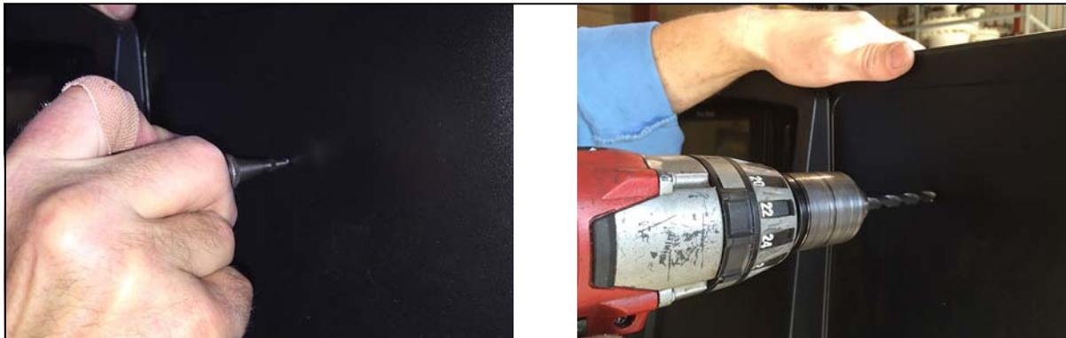
6. Remove any burrs around hole being careful not to damage the any paint/graphics present on the front of the door.
