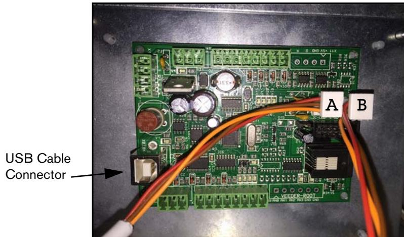
Route and fasten excess wire of the wiring harness using cable clamps (not included) as necessary to prevent possible damage to the harness during routine dispenser maintenance.
