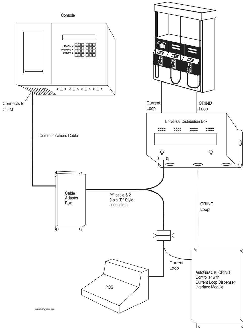
**Figure 7.** AutoGas 510 CRIND Controller with Current Loop Interface
