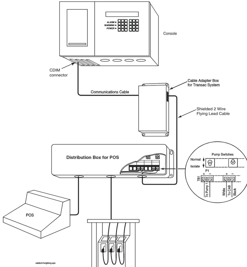
**Figure 5.** Transac Series Current Loop Interface
