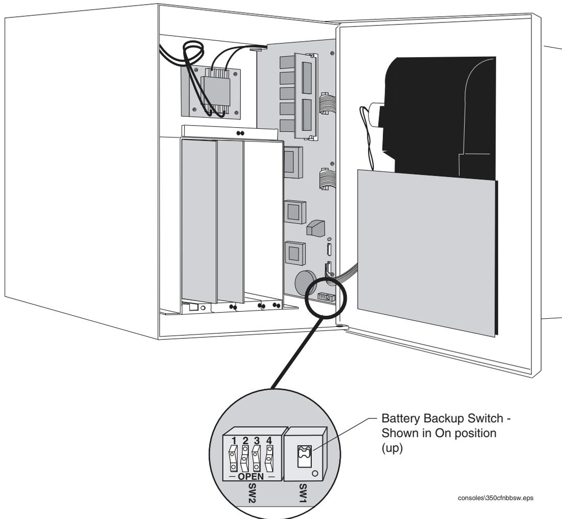
**Figure 1.** ECPU Board Battery Switch ON (SW1)
