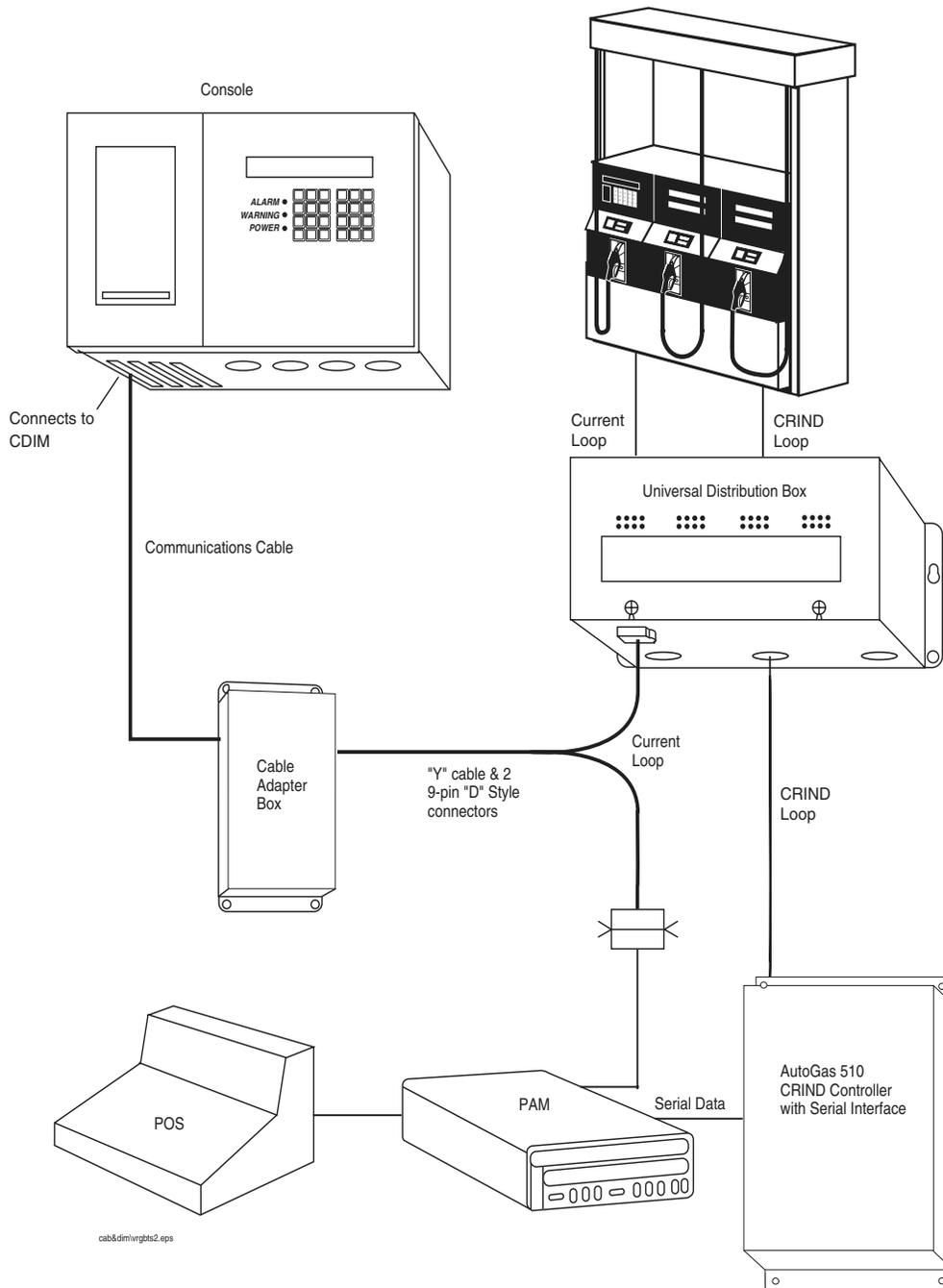
Figure 8. AutoGas 510 CRIND Controller with Serial Interface
