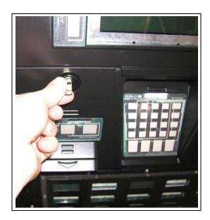
**2** Open the printer door and pull out the slide completely.
