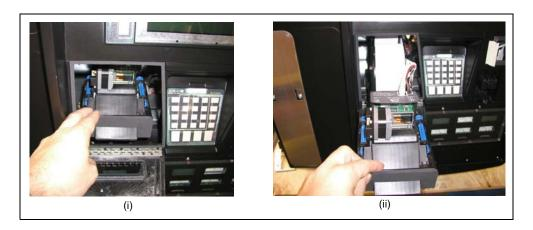
**3** Pull the empty paper spindle from the cable clamp. *Note: The unit is shipped with the spindle held by the cable clamp.*
