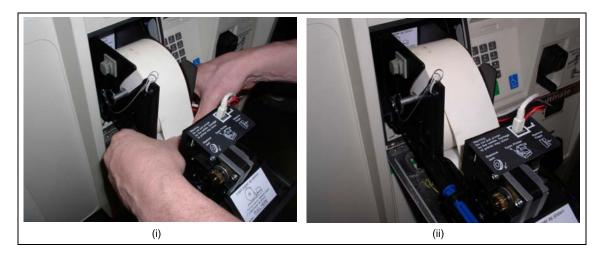
**7** Push the printer slide back in and feed the paper through the slot. Close the printer door and turn the key to the right to lock it.
