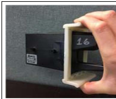
To install the dismount sensor clamp, apply pressure with both the thumb and the fingers to bend the clamp to fit the HCRS into the clamp as shown in [Figure 38](#).
