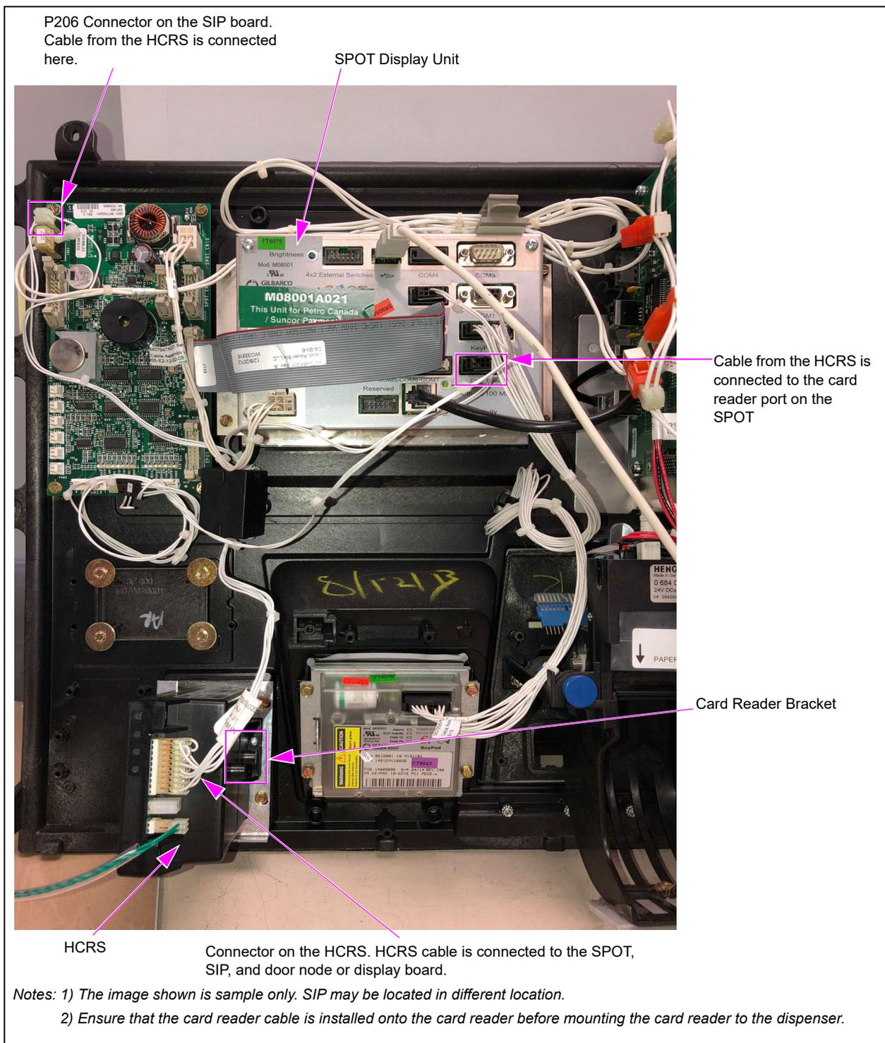
P206 Connector on the SIP board. Cable from the HCRS is connected here.
