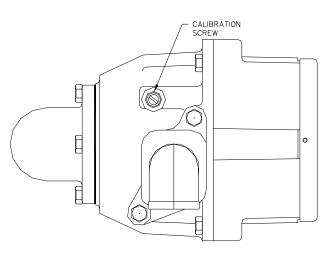
For new style meters, start with the screw turned all the way in clockwise. For gasoline calibration, turn the screw approximately two full turns counter-clockwise. For diesel, turn the screw approximately two additional full turns counter-clockwise.
