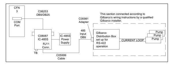
SW1 and SW2 of the IC-485S Converter should be set to DCE and T-on R-on. Connect the power supply to the power jack of the converter and plug the standard outlet cable into an available outlet, preferably on a backup power supply or power conditioner.
