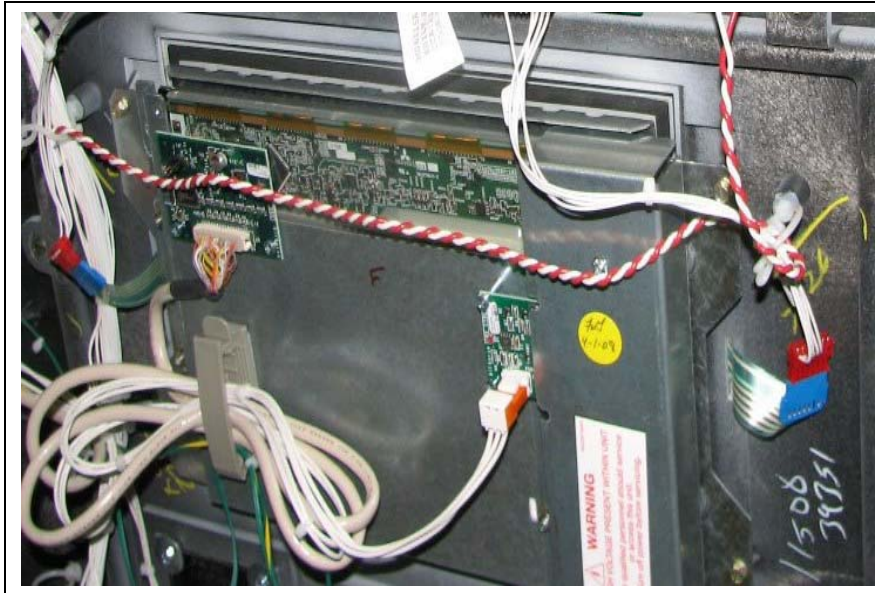
Figure 16: CRIND Cables on E-CIM
