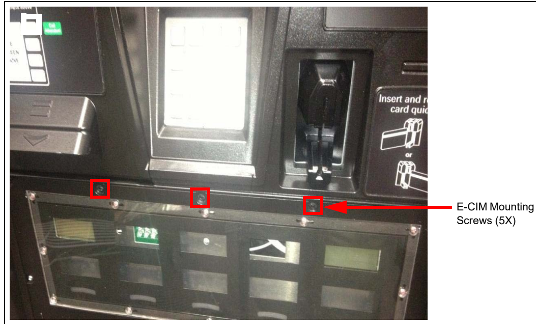
Figure 10: Loosening and Removing E-CIM Mounting Screws
