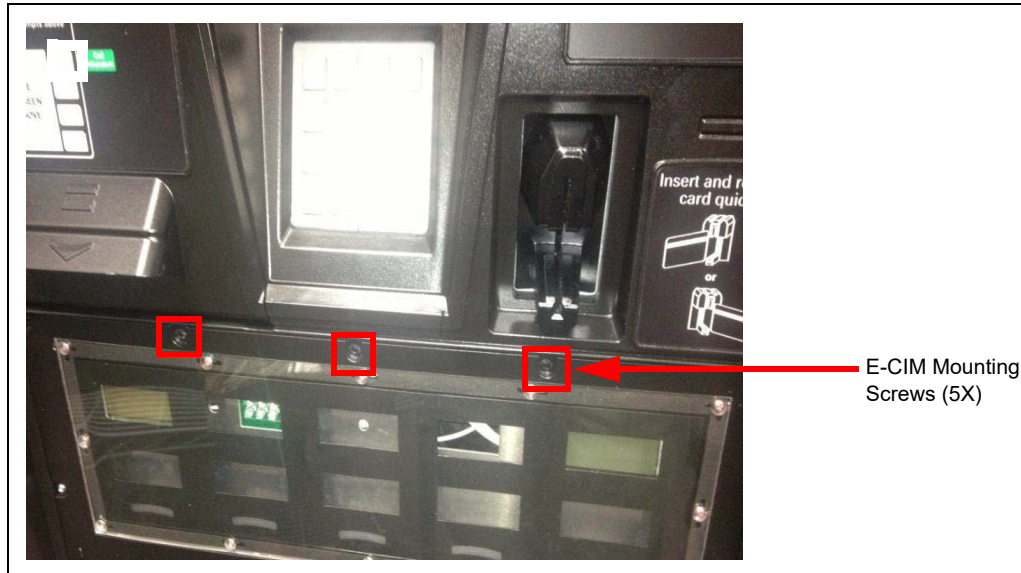
Figure 3: Loosening and Removing E-CIM Mounting Screws
