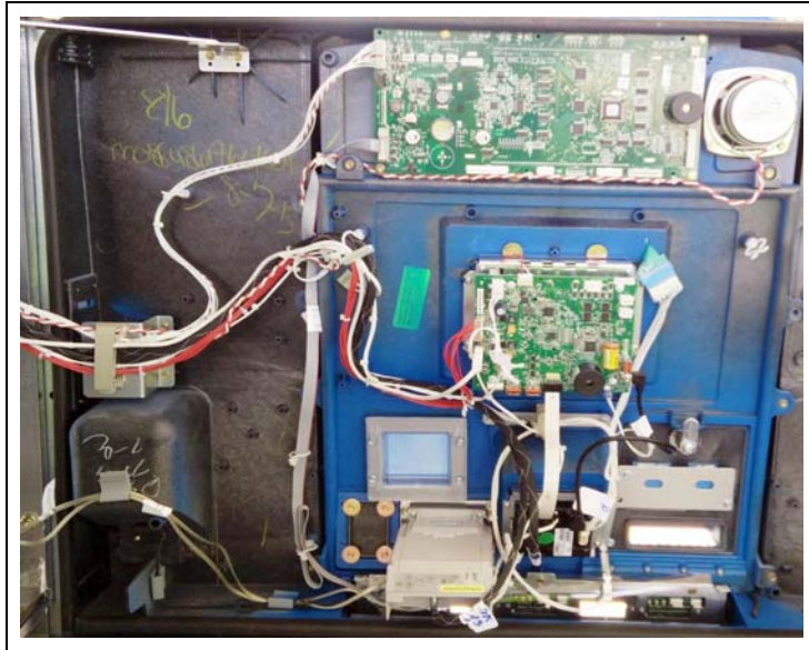
Figure 8: Cable Connections on Display Assembly
