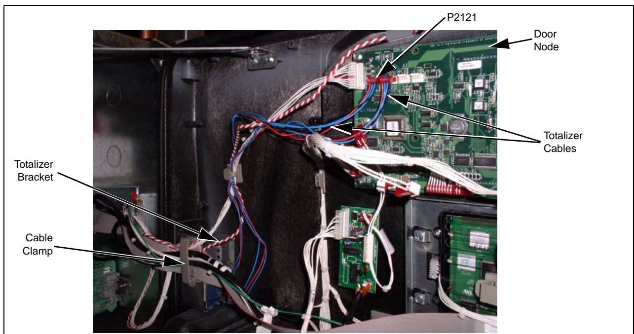
Figure 4: Installed View of the Totalizer Assembly with Cable connections
