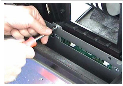
Figure 4: Securing PPU Board
