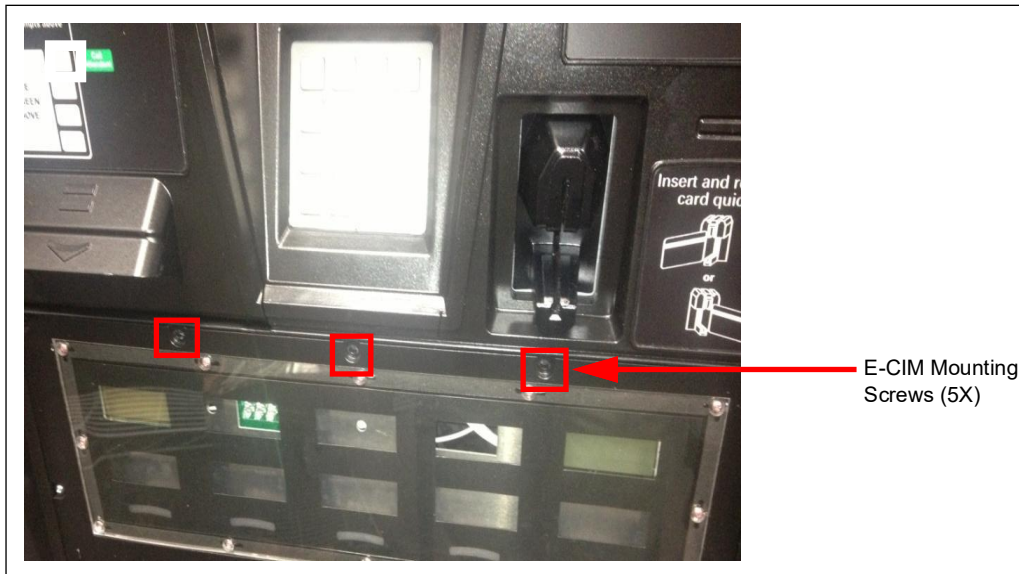
Figure 3: Loosening and Removing E-CIM Mounting Screws
