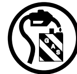
Collect fuel in approved containers.
