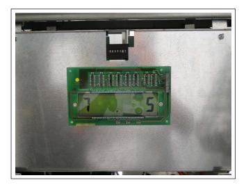
2 After the required can size is displayed, remove the nozzle and switch on the pump handle. This selects the can size for calibration.
