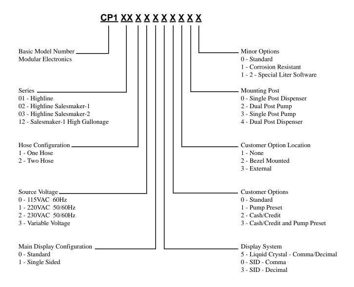
Thirteen digit electronics model number is stamped on plate attached to bottom of electronics module.
