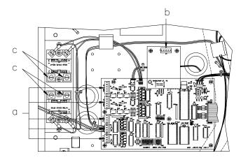
9. On one of the display panels, pull off the ribbon cables (a) from the LCD Display PCBs and the power cables (b) from the LED Backlight PCBs. Remove one end of the ground braid cable (c) from the display panel. Remove the two screws (d) from one of the support brackets. Be careful not to let the display panel fall while removing the support bracket. Slide the panel away from the remaining support bracket and pull it out of the cabinet.
