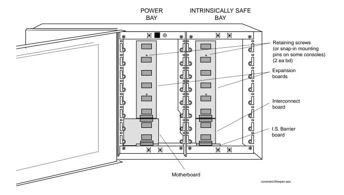
Figure 1. Expansion Board installation
