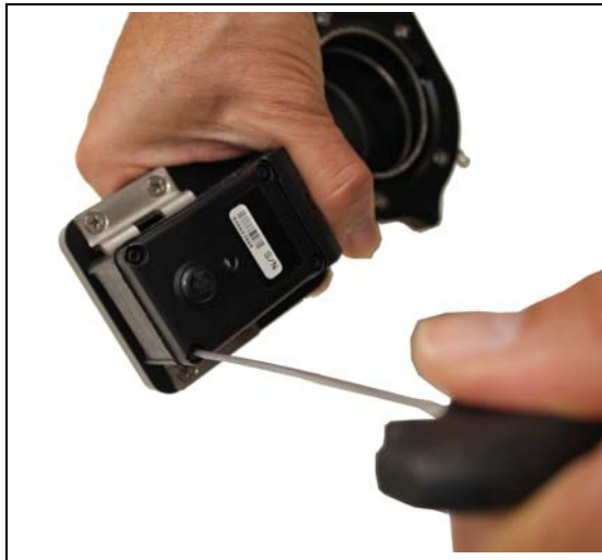
Figure 6: Removing the Top Cover Screws
