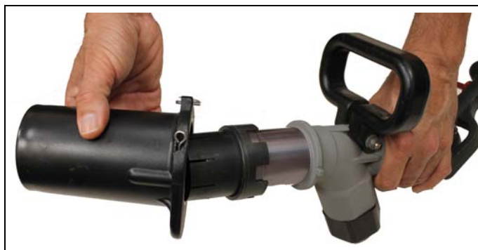
Figure 3: Removing the Original Wiggins Cover
