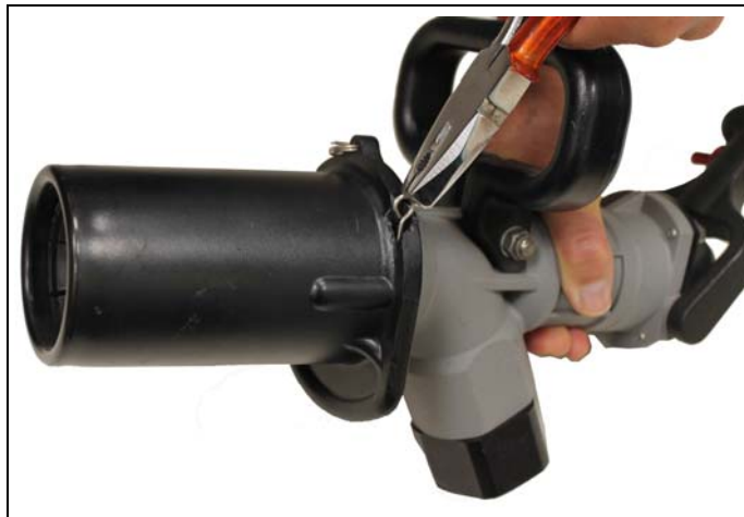
Figure 2: Removing the Pins from the Wiggins Cover
