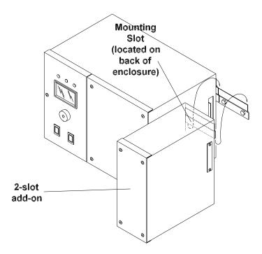
Figure 2 Hanging the 2-slot add-on on the Interlocking Rail
