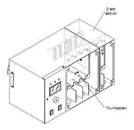
Figure 3 Securing the 2-slot add-on
