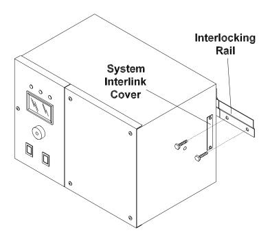
Figure 1 Removing the System Interlink cover and mounting the Interlocking Rail
