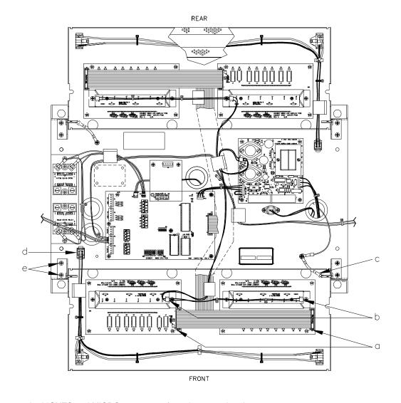
9. Disconnect the LIGHTS and MICRO connectors from the power bracket.
