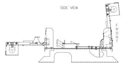
Feed the DC cable up through the platform bushing (a). The DC cable is a 4-conductor gray cable with red, green, white, and black wires terminated to a 5-position connector. It is part of the DC conduit assembly. Attach the DC cable to P1 (b) of the RS-485 I/F PCB.
