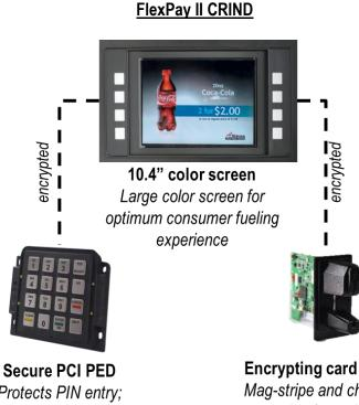
Secure PCI PED Protects PIN entry; provides PCI and EMV compliance
