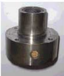
Bottom-end housing with bearing and breather
