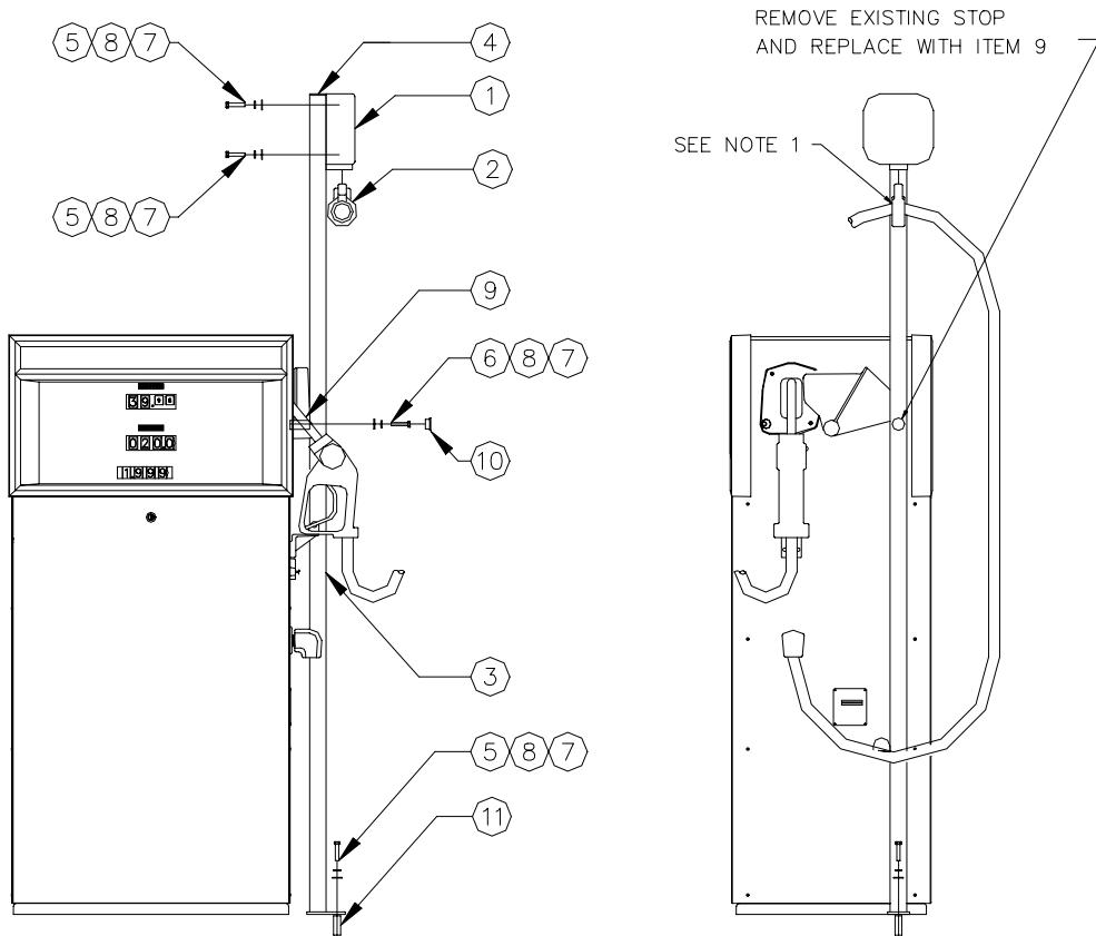
Complete High Hose Retriever installation requires a support post kit and a hose clamp/spring reel kit.
