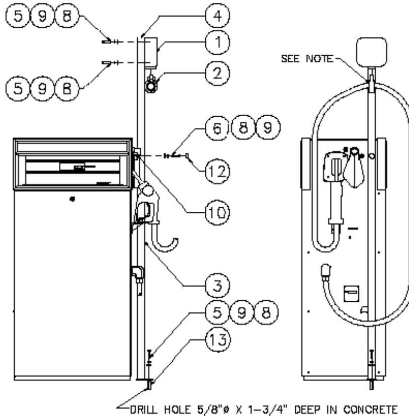
NOTE: Clamp should be positioned so that hose does not touch the ground when nozzle is hung in nozzle boot.
