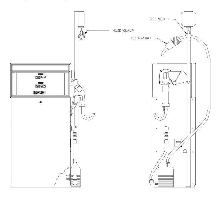
NOTE: Assemble supplied hose retractor clamp to high hose retriever reel assembly. Clamp should be positioned so that hose does not touch the ground when nozzle is hung in nozzle boot.
