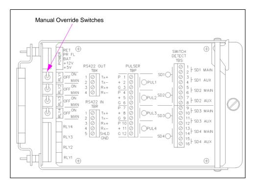
If this manual-override procedure does not work, chances are the power supply or the relays in the PCU are bad, and your only choice at this point is to replace them.
