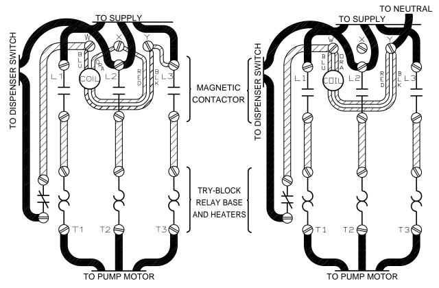
NOTE: COIL ABOVE IS WIRED FOR 220V TO PUMP MOTOR, 220V TO DISPENSER SWITCH
