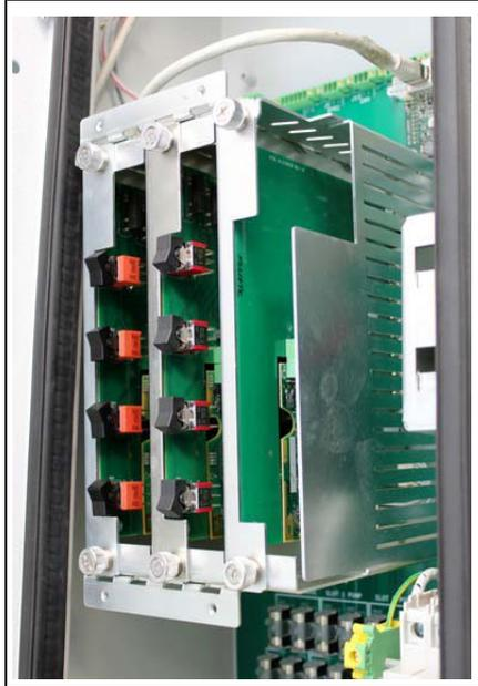
*Note: If you are adding a mechanical interface, it may be inserted into slot 1 or slot 2 only.*
