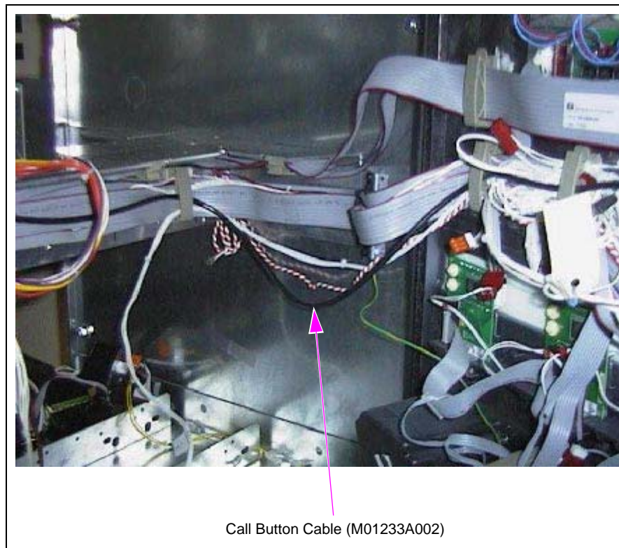
Figure 45: Encore Top Electronics Shelf with Call Button Cable Run
