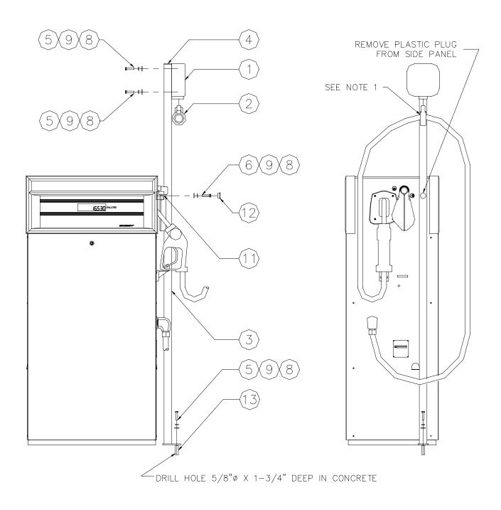
NOTE 1: Clamp should be positioned so that hose does not touch the ground when nozzle is hung in nozzle boot.
