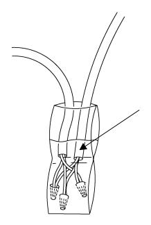
All wiring, including outer jacket should be completely submerged in epoxy.
