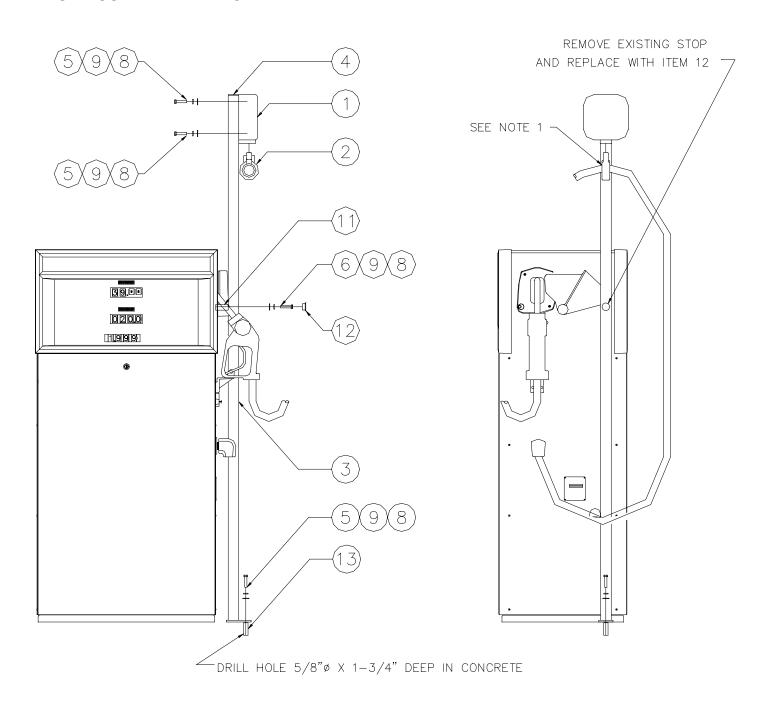
NOTE 1: Clamp should be positioned so that hose does not touch the ground when nozzle is hung in nozzle boot.
