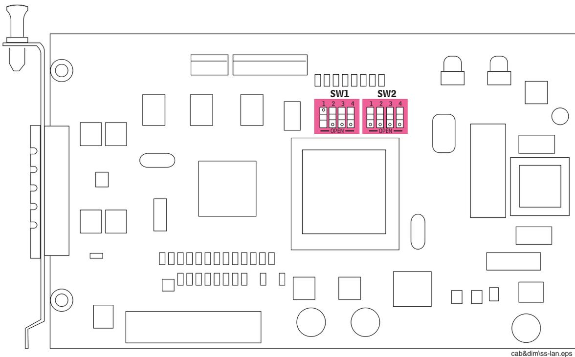
Figure 1. Dip Switch SW1/SW2 on SS-LAN Interface Module
