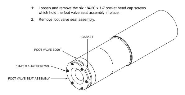
3. Use a putty knife to remove any residual gasket material left on the foot valve body.
